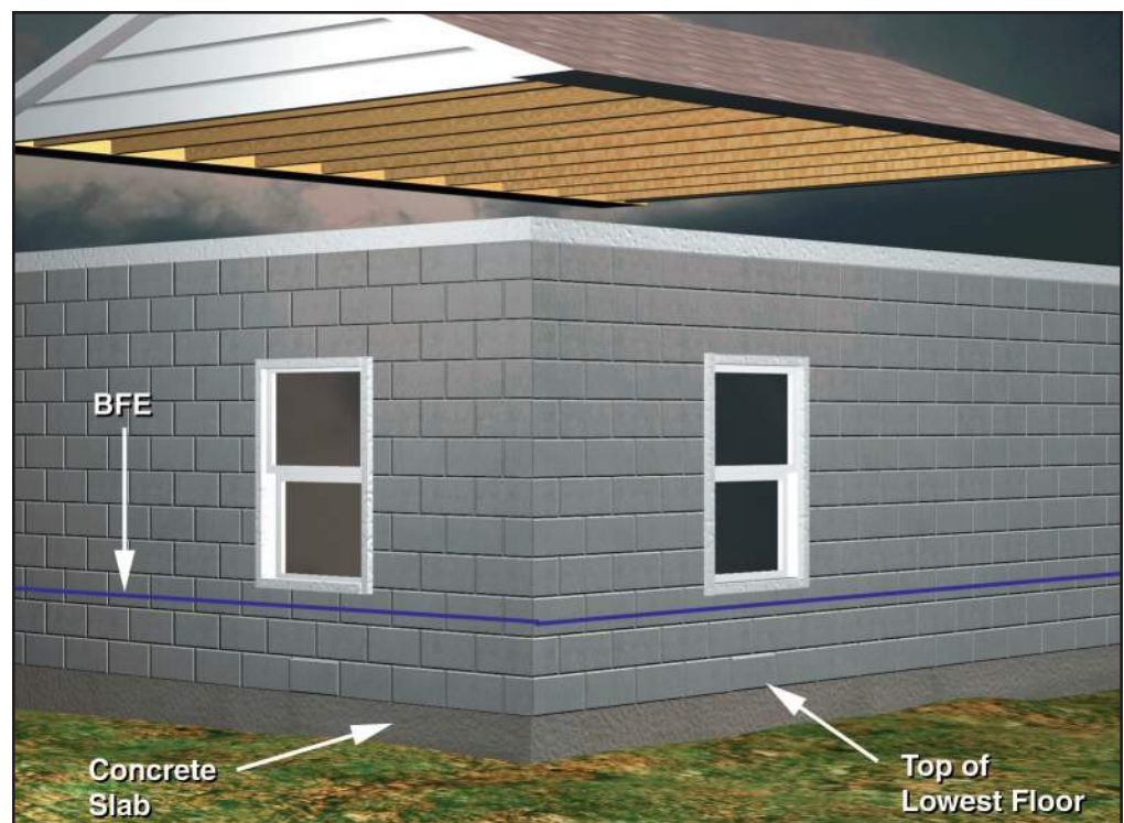
Figure 10 The first step in Technique 1 is removing the roof.
